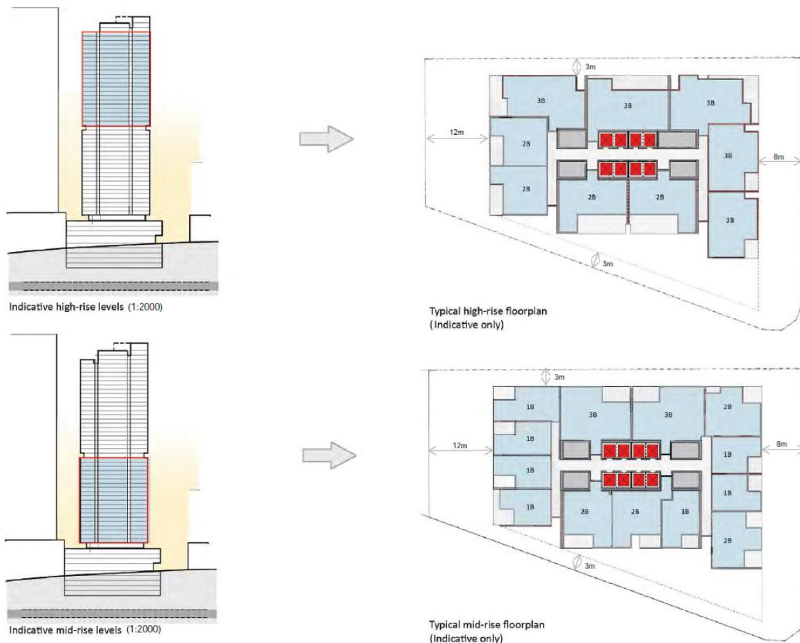
Figure 7: Typical tower floor plate (indicative only) source:
